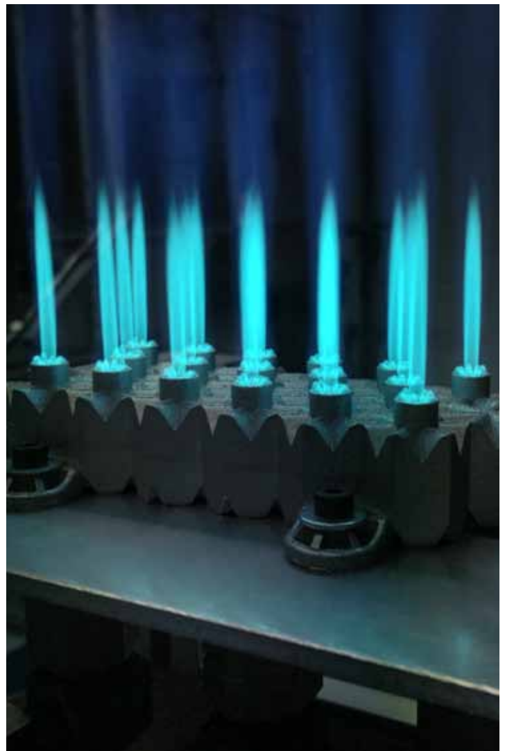
AM printed LINDOFLAMM burner in action
